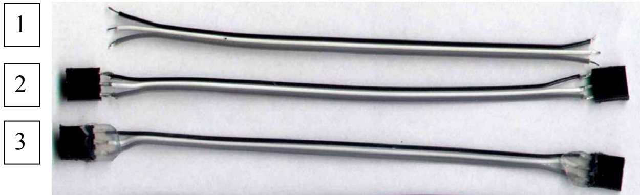
Figure 31. F3W3F3 IR DETECTOR CABLE: CIRDLF (6 inches), CIRDRF(6 inches), CIRDB (optional, 3 inches).
