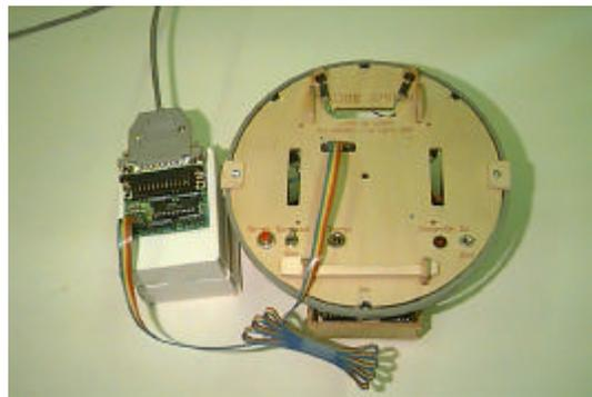
Figure 5 This Photograph shows the gray serial cable from a PC COM port mating with the D-25 connector on the communications board (com-board = MB2325 = the exposed circuit board sitting on the white boxes). The multicored 6-wire serial cable attaches to the male header on the com-board and into the serial slot on the TJ™ plate. Note the same color orientation of both ends of the 6-wire cable for the configuration pictured.
